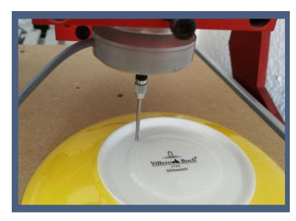
With a suitable 3D probe or tracing pin, non-planar surfaces of workpieces or even entire machine tables can be scanned and stored as a measurement table. Subsequent machining with engraving or milling can then take the measured values into account and project the data onto them.
