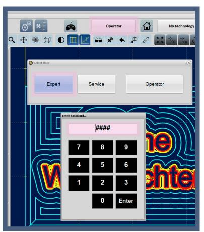
and execute jobs and initialize the machine. The *expert* may set up new jobs or modify existing ones and make all job settings, and the *service employee* has access to all functions and settings of the machine and the system.
