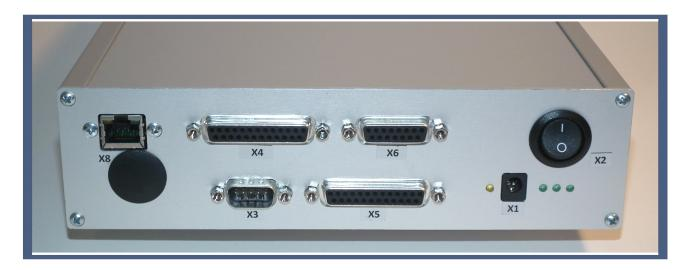
The axis controller is connected with a standard CAT cable and can be connected either directly to the control computer or via one or more switches in a network. This makes it easy to operate even in remote locations.
