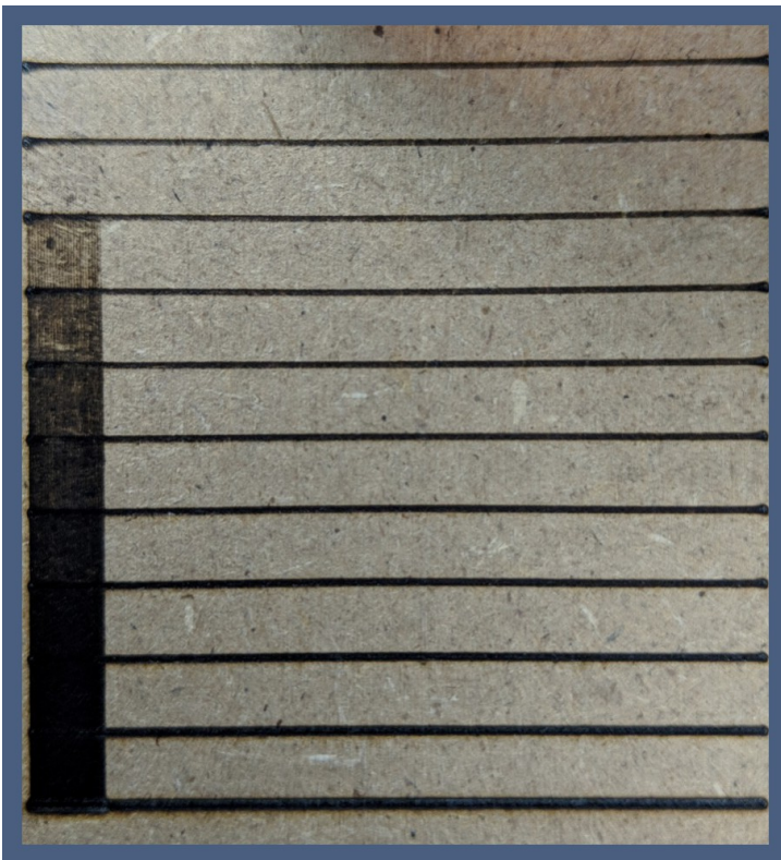
Image: Laser speed and greyscale test
