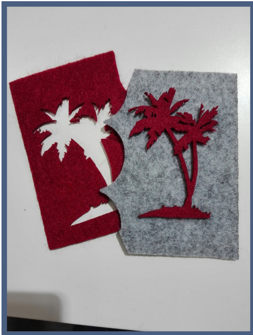
Picture: Cut felt with 4 passes and without burn edges
