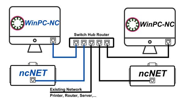
By default, *WinPC-NC* always connects to the first available *ncNET* module in the network. To enable an exact assignment of the *WinPC-NC* instance to the corresponding *ncNET* module, the checkbox "Connect to *ncNET* from LIC file only" must be activated in the parameters under Basic Settings-Ports. The change to the settings is applied by clicking on Save. *WinPC-NC* is then closed and restarted.
