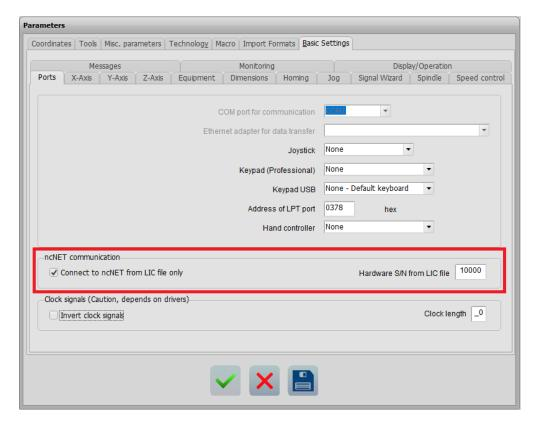
**WinPC-NC** now always connects to the **ncNET** module whose serial number is specified in the WinPCNC.LIC license file. This number is also displayed in the "**Hardware S/N from LIC file**" text box in the parameter dialog for checking purposes.
