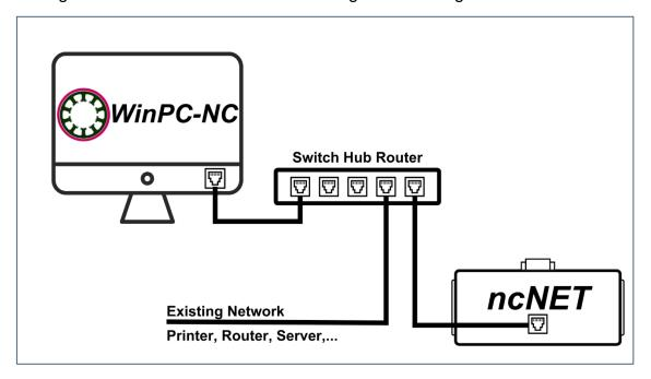
We offer a suitable network switch with 5 ports that has been tested for use with **WinPC-NC** in our online store:
