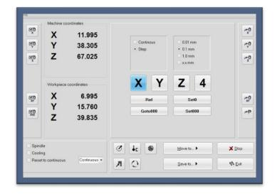
In step mode, an increment of 0.01 or 0.1 or 1 mm can be defined and *WinPC-NC* moves the set distance with the active axis each time the upper encoder wheel is turned. This allows precise positioning and distances to be moved and the axis movement takes place with every noticable snap-in position.
