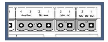
The ready or emergency signal on clamp X3, contacts 1/2, activates the three power drivers for the motors and also acts as enable signal for the relays. The signal is routed to the enable input of the power drivers and can therefore be used as an emergency signal or as a contact of a protection hood.
