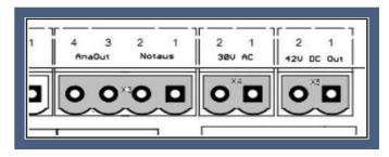
When decelerating, a stepper motor acts as a generator and supplies current back to the power supply. This will temporarily cause the supply voltage to increase significantly. To prevent rising above 45VDC, an electrolytic capacitor can be connected to clamp X5 in addition to the capacitor in the power supply.
