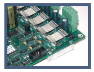
The version **Step3S HT** is designed for ambient temperatures up to 70°C and is equipped with passive heat sinks on both top and bottom side. A fan should be used in a similar way than on the standard version.
