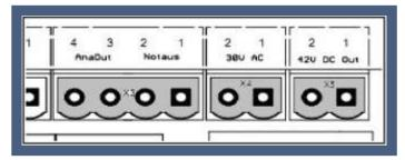
The stepper motor board **Step3S** can be supplied with either AC or DC voltage. When using DC power, the lower threshold is 12V~ while the upper threshold is 30V~. For DC power the thresholds are 15V= and 42V=, the polarity is irrelevant.
