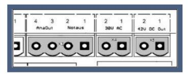
**Step3S** can convert a PWM input signal (min. PWM frequency 200 Hz) to an analogue output signal. Many frequency converters accept such a signal as reference value for the rotational speed of synchronous or asynchronous main spindle motors. Consult the manual of your converter to see how the reference input has to be parameterised.
