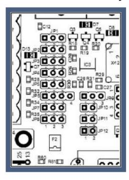
Depending on the signal level to control the relays, it may be, that the behaviour of the relays is inverted compared to the driving logic. Additionally, during power on or boot up of the PC the relays may be switched unintended. With JP12 closed, the control signals for all three relays are inverted.
