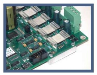
The *HT* version for ambient temperatures up to 70°C is equipped with a 10mm thick aluminium heat sink on the bottom side. This heat sink has to be mounted to the bottom plate of the case with its full surface. This ensures optimal heat conduction.
