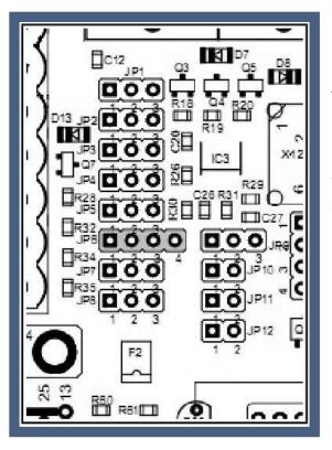
If set to position 3-4, the signal coming from Pin14 is fed to the PWM logic and converted to an analogue signal with 0-5V or 0-10V range. If a jumper is set to position 1-2, Pin14 controls relay 2. When both jumpers are set, Pin14 is fed to the PWM logic and relay 2 is switched automatically depending on the PWM value.
