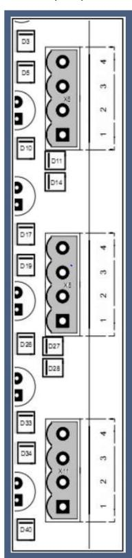
**Step3S** is designed for 2-phase stepping motors only. It can be used with both bipolar and unipolar motors. If no datasheet is available to your motors, you have measure which connectors belong to which winding of the motor.
