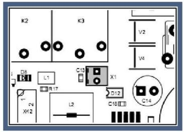
On the connector X1 5VDC are supplied for the fan mounted to the side of the board. This fan can be mounted on the upper or lower side of Step3S, depending on mounting situation and ventilation in the case. If a case with integrated fan is used, the air stream should pass the 6 drivers (IC's 1, 2, 5, 7, 12 and 17). The direction of the board's fan air stream should be adjusted in the same direction as the case fan. In this case the fan mounted to the board may be redundant.
