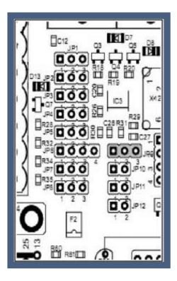
The PWM signal can be evaluated from pin 14 or pin 17. The mapping of the signals is done by jumpers JP2, JP3, JP5 and JP6.
