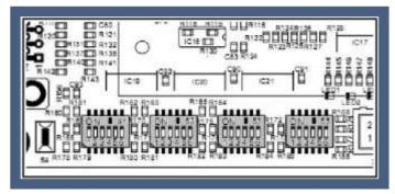
The stepping motor drivers support microstep operation. They produce a sinusoidal course of motor currents. The step width can be set individually for each motor with the left three DIP switches according to the following table.
