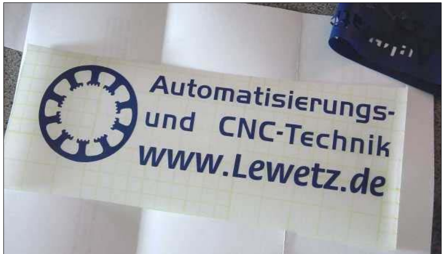
Sample for foil cutting with tangential axis
