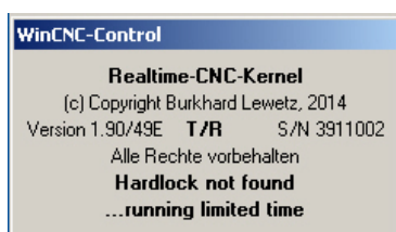
Display of the realtime module if the USB dongle has not been found
