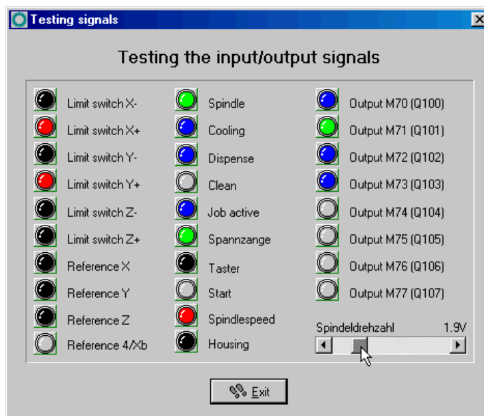
Special function SIGNAL TEST with LED displays of the most important inputs
