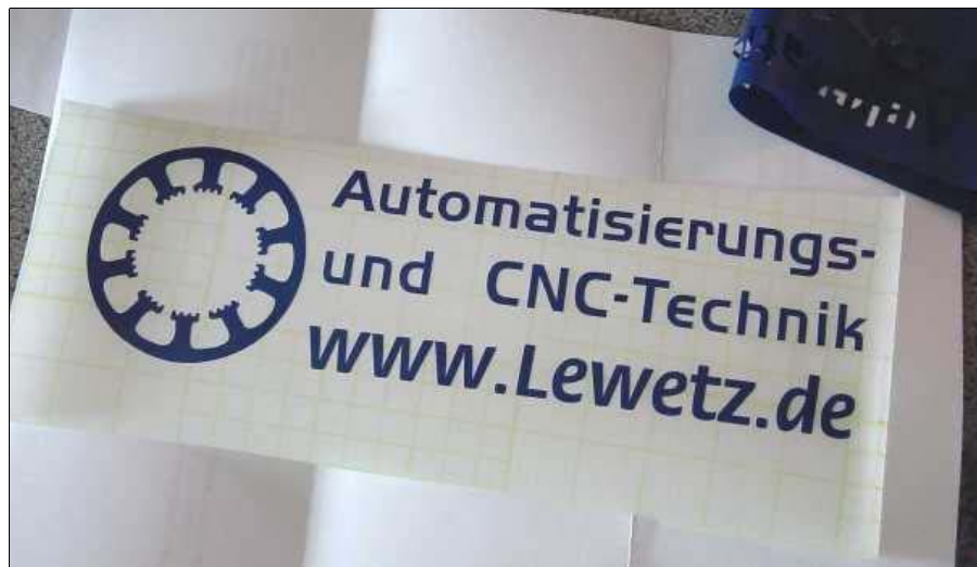
Sample for foil cutting with tangential axis
